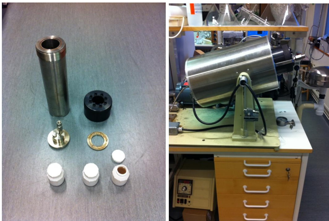
Figure 13. On the left the bomb and three samples opened. On the right, Parr pressure reactor 4841 assembled.
