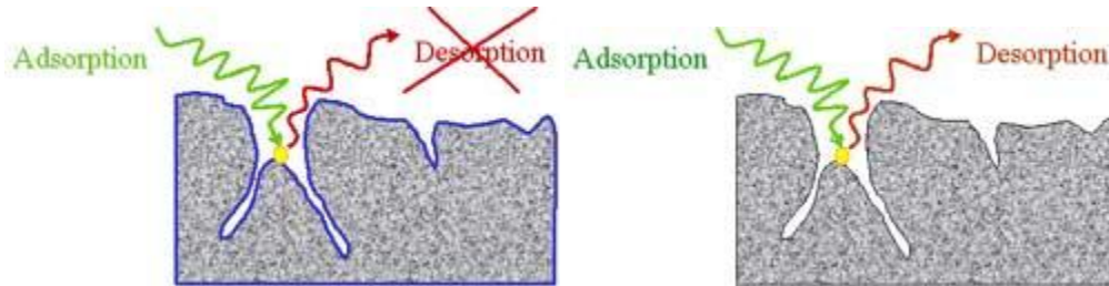
Figure 9. Sorption mechanisms of chemisorption and physisorption.
