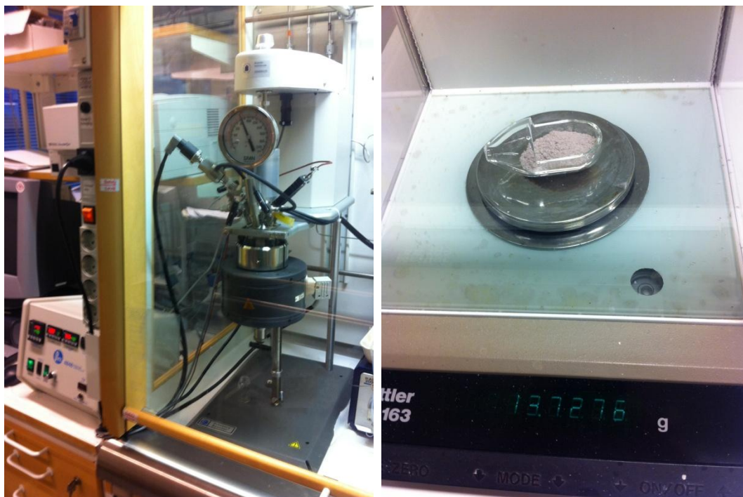
Figure 14. On the left, Parr pressure reactor 4848 and its controller unit. On the right, ash sample in the glass vessel in Mettler electronic balance.
